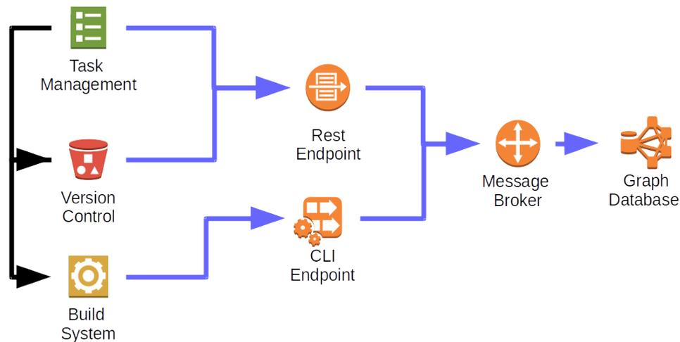
Figure 4.1: Illustration of the test setup. The black arrows illustrate the flow of inter-tool messages. The blue arrows illustrate the framework messages and endpoints.
