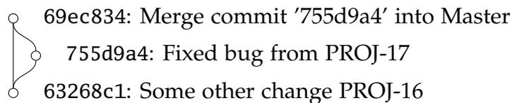
Figure 4.4: Illustration of the two branches *master* (left) and *development* (right). A change is made at development and merged back to master.
